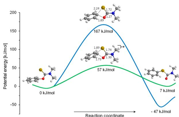
**Figure 3.** Schematic potential energy profile comparing the G4MP2 calculated reaction coordinates for the thermal NKR (blue) and the oxidative NKR (green). The reactant is set at 0 kJ/mol for each reaction; the energetic separation between the two should in reality be the ionization energy of  $\sim 750$  kJ/mol.
